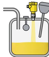
With its compact design and process fittings down to ¾" thread, VEGAPULS 64 can be used very effectively on small tanks and containers.
